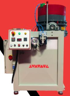
The SM Series machines feature a unique rotary base process chamber and fixed chamber walls. After each cycle, the entire chamber tilts to an angle of 140 degrees, effortlessly transferring the processed material to the VE series vibratory separator. This innovative design eliminates cumbersome manual handling, maximizing productivity and minimising downtime.
