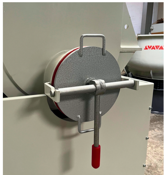
QUICK RELEASE DISCHARGE
