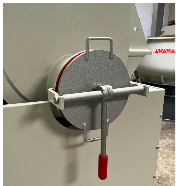
QUICK RELEASE DISCHARGE
